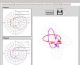
Radiation pattern of the antenna, whose representation may be in cartesian, polar or threedimensional form. Measurement of intensity, frequency and angle of interfering signals, which are generated by GSM and UMTS stations, Wi-Finetworks or television broadcasters.
