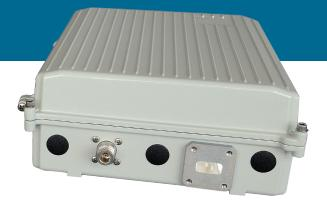
Like the Up Converters, also the Down Converters are generally proposed in the version of waterproof box for outdoor environments. This allows installations closer to the antenna, minimizing losses due to wiring. The Down Converters are powered via the output connector of the IF signal and they internally contain PM Microwave local oscillators, which boast excellent stability and spectral purity.
