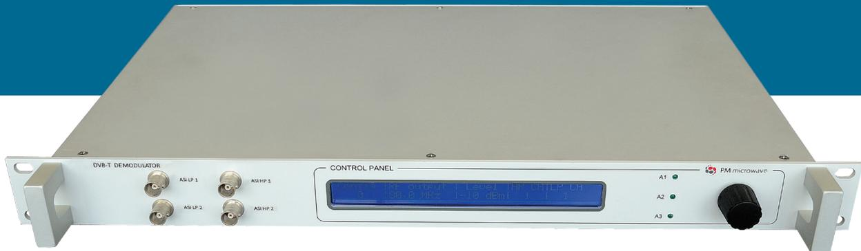
The DVB-T/H demodulator allows to receive 2 IF signals coming from a diversity receiving system in the 50 ÷ 850 MHz band, thus making possible a robust demodulation even at low SNR values. The diversity DVB-T/H demodulator supports all demodulation modes defined in the ETSI DVB-T standard (EN 300 744). The ASI output stream is compliant with EN50083-9 standard.
