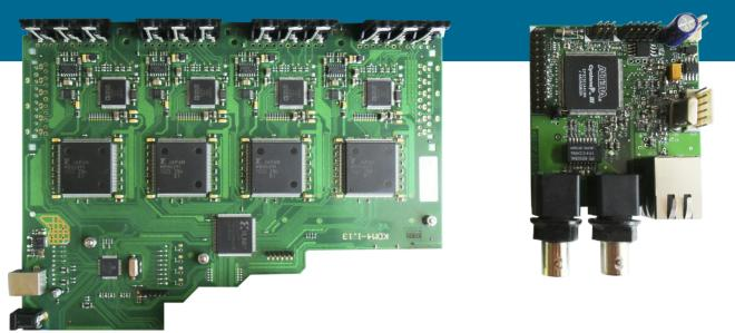
The MPEG-2 encoder with IP output can encode up to 4 audio / video inputs and provides a UDP / IP output stream containing the Transport Stream of the 4 channels. It is proposed as a series of modules that allows for easy integration into existing solutions.
