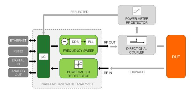
▲ External RF directional coupler and detector are available as an option in order to make even measures of return loss.
