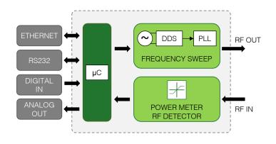
The Narrow Bandwidth Analyzer is a compact and versatile device which allows to measure the frequency response of a generic 2-port network. It mainly consists of a frequency sweep generator and of an RF logarithmic detector that captures the  $S_{21}$  response of the device under test.
