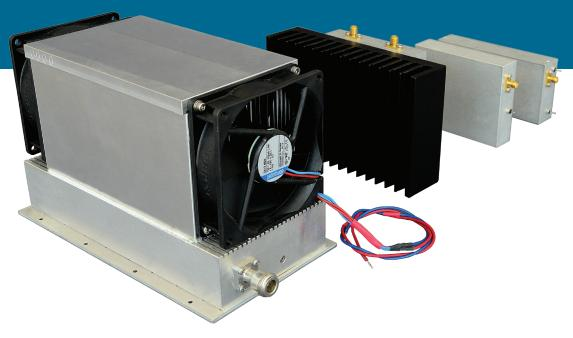
The power amplifiers that PM Microwave includes in its products portfolio are able to cover applications that require signal powers up to 50 W. These are Class A amplification modules with excellent linearity, and are therefore suitable to work with digital modulations of high order and complexity. Depending on the model, the devices can be equipped with passive or active heat sinks. All modules are tested in temperature to ensure the maximum reliability of operation over time. The RF powers and
