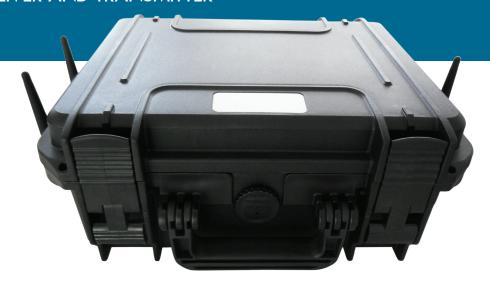
The DVB-T REPEATER is a compact and transportable solution to extend the range of a DVB-T link without the need of a coaxial cable. The RF frequency can be selected in the ISM band ( $2400 \div 2500 \text{ MHz}$ ). The 2-way diversity receiver allows to reach great performance even in case of mobile links. The rechargeable and easy-to-be-replaced battery allows to reach an autonomy between 5 and 7 hours.
