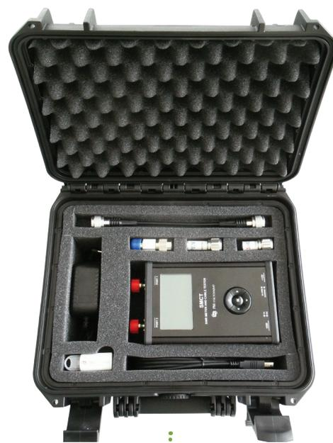
The hard transit case protects the SMCT and its accessories, i. e., the calibration kit, the battery charger, a USB cable and key (with SMCT GUI software).
