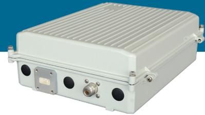
The analog transmitters proposed by PM Microwave are devices designed to be used both in analog and digital broadcasting. They are available in both 19" rack for indoor use and waterproof box for outdoor use. The available versions work in the 7 GHz, 10 GHz, and 14 GHz bands, with output powers of 500 mW (+27 dBm) or 1 W (+30 dBm).
